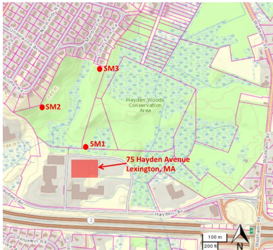
Figure 1. Area plan showing building location, nearest residences, and proposed sound monitoring locations SM1, SM2, and SM3 75 Hayden Avenue, Lexington, MA
